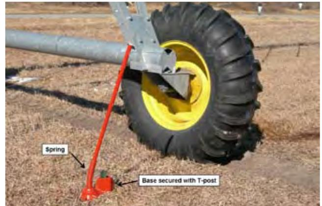
**Figure 8.** Commercially-available drive-over post used in conjunction with a single-strand high-tensile wire.
