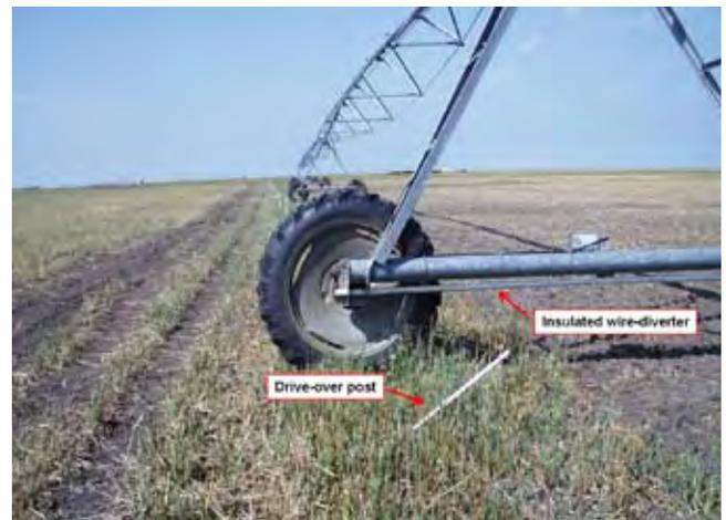
**Figure 9.** Pivot completing crossing of fence with drive-over posts. *Note:* The angle of the fence is offset from the pivot to ensure that only one or two towers are in contact with the fence at any time.
