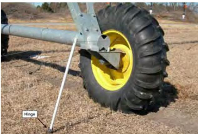
**Figure 7.** Drive-over post used in conjunction with a single-strand high-tensile wire. *Note:* Drive-over posts should be installed within 2 to 5 feet of the tower wheel.
